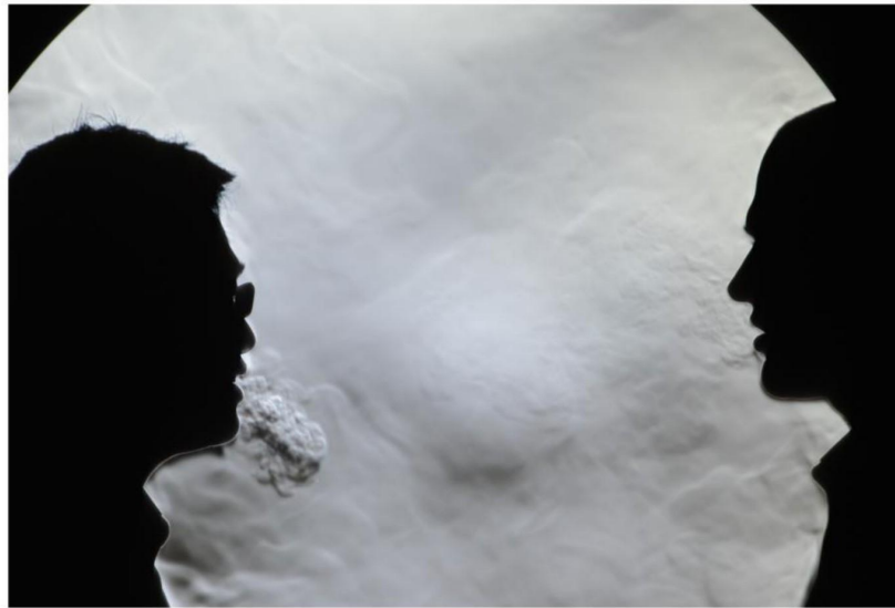
Figure 5. Schlieren image showing the interaction of two exhaled airflows between two people (reproduced from https://journals.plos.org/plosone/article?id=10.1371/journal.pone.0021392 , CC BY 4.0, https://commons.wikimedia.org/w/index.php?curid=90043870 (Tang et al. 2011))
