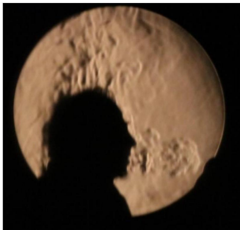
Figure 9. Schlieren photograph of a person talking. Notice: (i) the cone-shaped turbulent exhalation jet emanating from the mouth; and (ii) the vertical thermal plume passing over the
